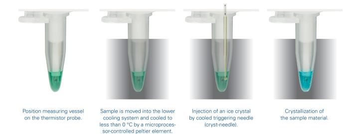
At the beginning of the measurement, the sample is supercooled in the lower cooling system. The freezing process of the sample material is released in a controlled manner by injecting an ice crystal using the release/triggering needle.
